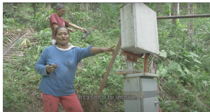
Figure 2. Another barangay volunteer shows how to use the PHIVOLCS landslide sensor in Saint Bernard, Southern Leyte (ACCORD, 2015)
